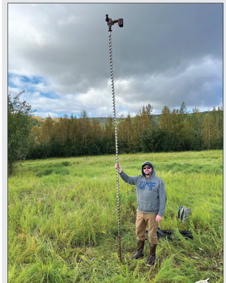
Electric drill with auger lets us look for permafrost in the upper 5 m of soil.
